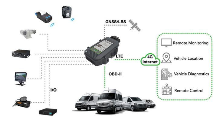
The VT310 offers a perfect solution to fleet management. Extensive I/O can be connected to a variety of devices on the vehicle via RS232. With low power LTE CAT-M/1 connectivity, the tracker is continuously connected to the vehicle and sends vehicle location, mileage, operation status, driving behavior, etc. to the remote management platform over 4G network.
